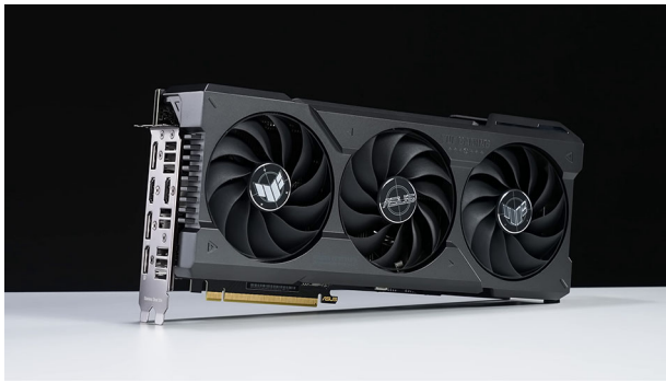
Fig. 1 A part of the body of a possible AI system—an example of the graphics processing unit (ASUS TUF RTX4070 Ti SUPER). Attribution: 极客湾 Geekerwan, CC BY 3.0 < https://creativecommons.org/licenses/by/3.0/ >, via Wikimedia Commons.
