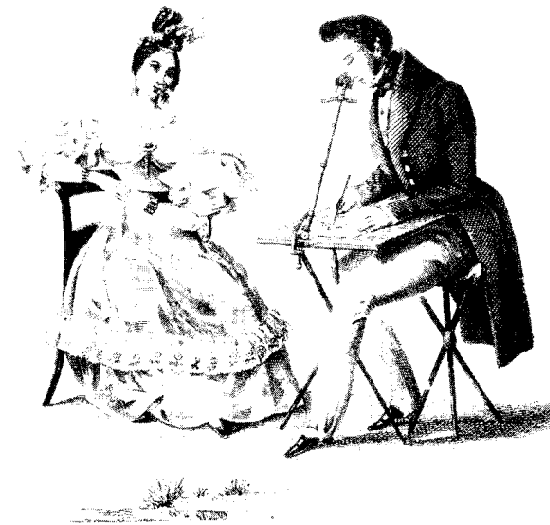
Figure 2-4. The camera lucida consisted of a lens arrangement that enabled the artist to view subject and drawing paper in the same "frame," and thus simply outline the image that appeared to be projected on the paper. ( International Museum of Photography, George Eastman House. )
